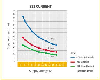
The 332 radar has taken the powerful feature rich experience from the low power AGD331. Using the latest power saving technology, the radar's design is a unique pulsed, frequency modulated transceiver linked to a 32bit ARM Cortex M4 processor. This helps deliver market leading radar performance while maintaining extremely low power usage.
