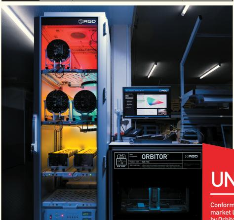
**Orbitor**™ and **Neptune**™ are bespoke sets of test equipment designed and developed by AGD Systems. They are dedicated to the testing of the 94X nearside signals and 100% of units manufactured at AGD are Certified by Orbitor.
