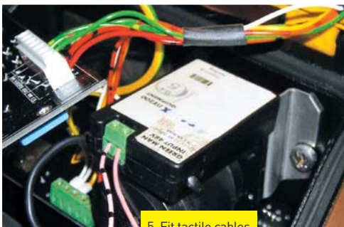
5. Fit tactile cables and slide module to position shown
